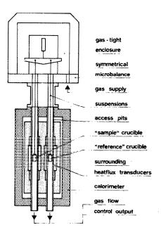
Fig. 1. TG-DSC schematic cross section
